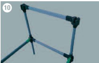
10 Repeat the build sequence with riser cups, 300mm legs and black rails on the front of the forth row. Connect this frame using green rails into 600mm legs into the back of the tiering block.
