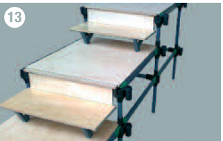
13 Deck bar adapters should always be located in the first and second nodes from the top of the row. This should be done for all rows after the first.
