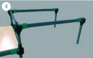
4 Then continue to build the second row using green Rails connected to 450mm Legs.
