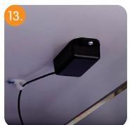
13. Built-in heat sensor will shut off power if a device overheats or if interior temperature reaches 32C/90F degrees to prevent risk of fire or damage to devices.
