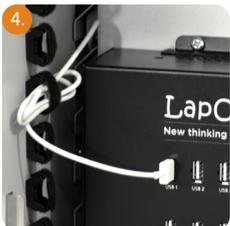
4. Individual velcro cable fasteners secure cables in place, organised and free from damage.
