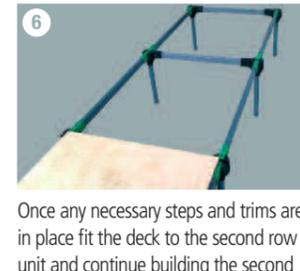
6 Once any necessary steps and trims are in place fit the deck to the second row unit and continue building the second row in this way until complete.
