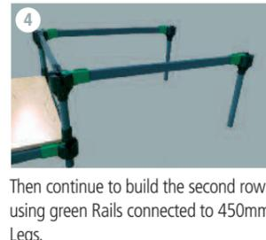
4 Then continue to build the second row using green Rails connected to 450mm Legs.
